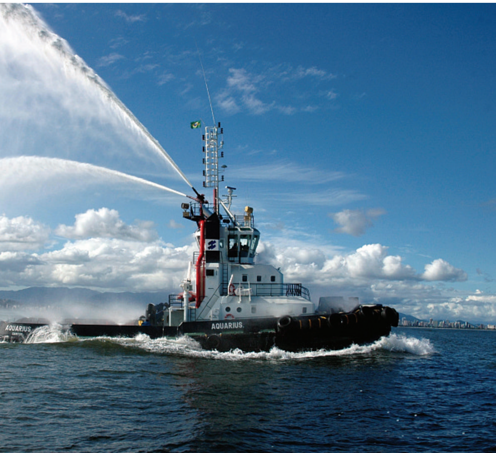
Above: The 72 ton Bollard pull tug Aquarius. The Aquarius is a Azimuth Stern Drive (ASD) tug-boat and was completed at our shipyard in Guarujá in 2006.
